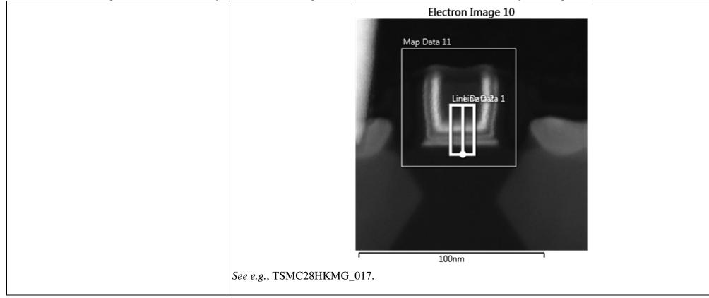
"forming an interfacial oxide layer over a channel region of said substrate, said interfacial oxide layer having a first thickness;"
