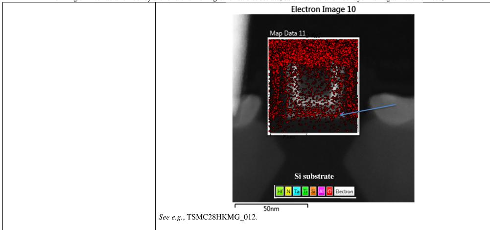
"forming an interfacial oxide layer over a channel region of said substrate, said interfacial oxide layer having a first thickness;"
